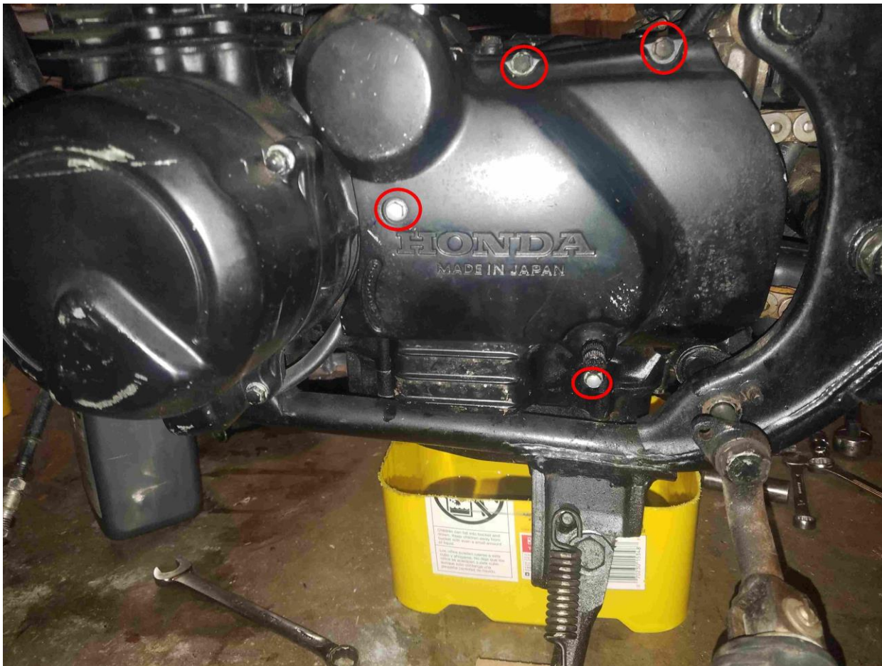
46. Replace the foot shift lever, slide it on the splined shaft before putting the 10mm bolt through it.
