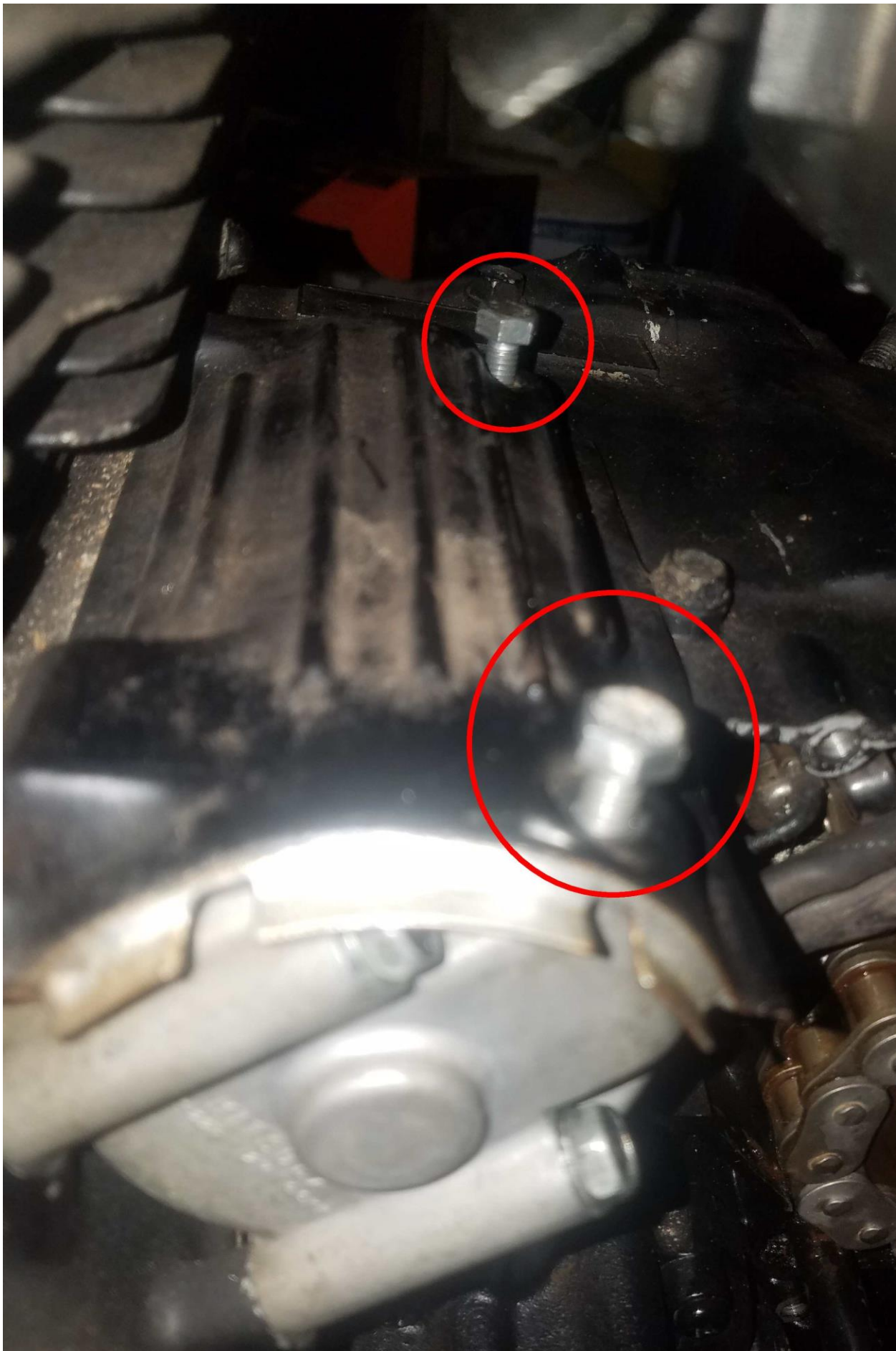
45. Replace the chain gear cover using the four 8mm bolts.
