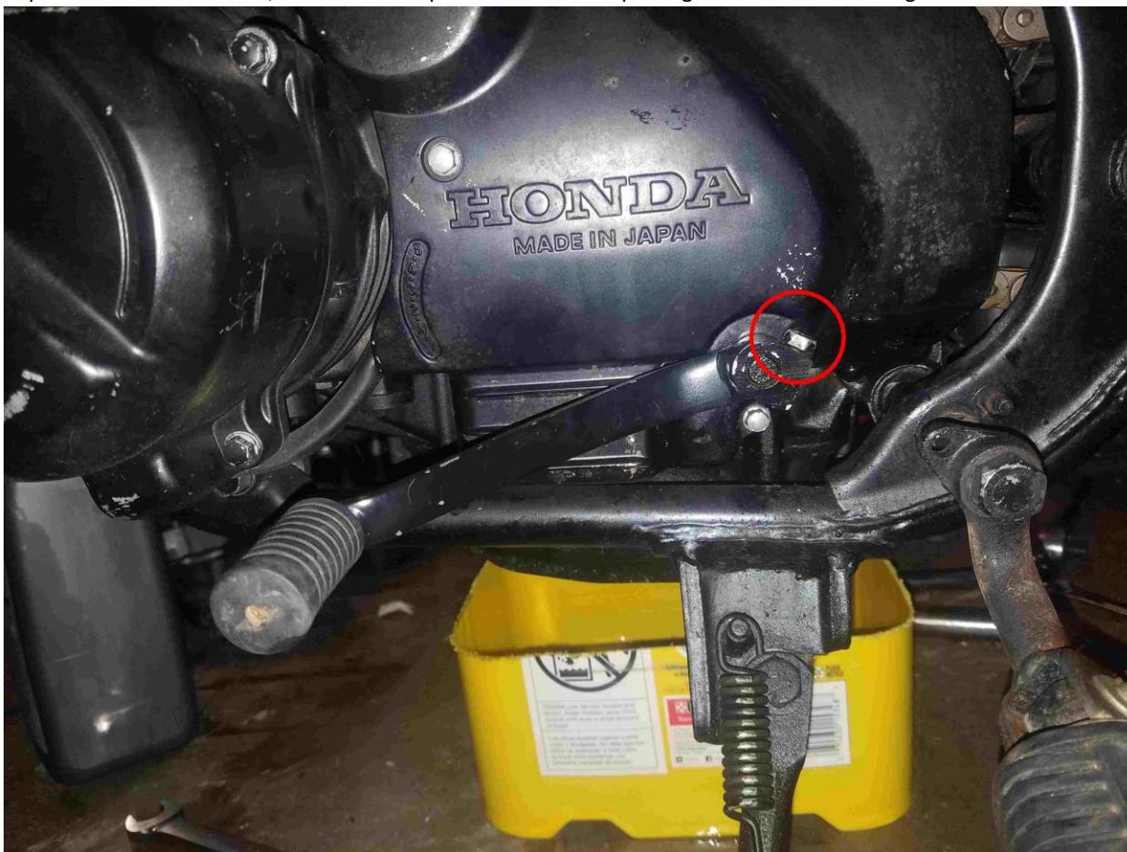
47. Replace the oil pan, use a new gasket if you don't know how old yours is. It is held on by ten 10mm bolts.
