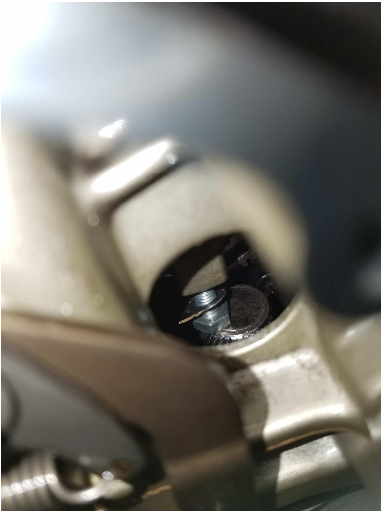
33. Time to re-insert the main shaft. Notice the order of the spacer and needle bearings that the clutch rides on.
